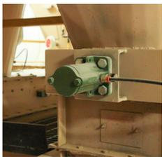
Moving feed efficiently out of the hoppers and limiting damage to the exterior walls requires the use of VMSAC 1200 Air-Cushioned Piston Vibrators from CVC.
